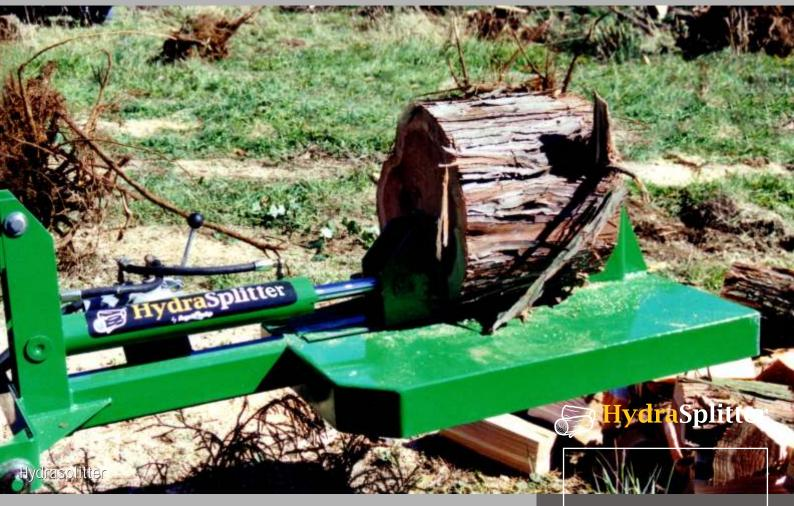
For larger tractors the Agriquip three point linkage mounted Hydrasplitter puts hydraulic power into use with unrivaled force. These splitters feature a simple, easy to use control valve with a convenient detent to return the ram quickly - ready for the next operation.
