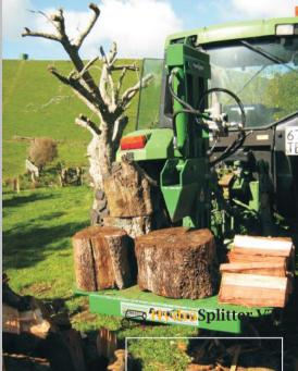
For larger tractors the Agriquip three point linkage mounted Hydrasplitter puts hydraulic power into use with unrivaled force. These splitters feature a simple, easy to use control valve with a convenient detent to return the ram quickly - ready for the next operation. The VTL can be used from a position sitting on the ground, to a point anywhere in the range of the tractors draft arm lit range, to suit any operator.
