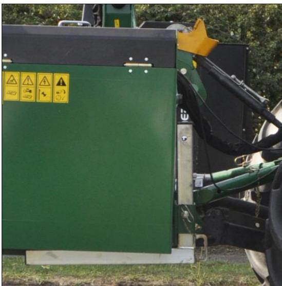
9. Raise leg stands to ensure they don't get damaged. Adjust check chains ensure the machine is secure and cannot swing from side to side.
