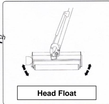
This option allows the flail head to follow contours of the ground without having to constantly control the angle of the head.
