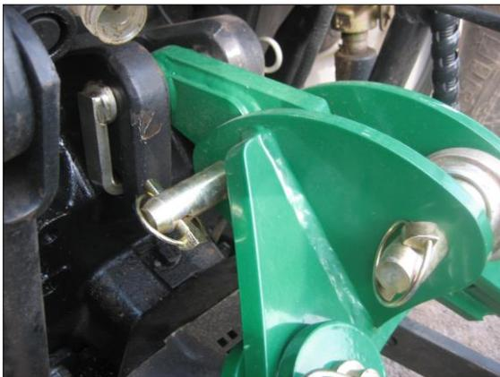
2. Fit stabiliser bracket into top link clevis and fit top link. The standard link comes with a Cat III hole plus a Cat III to Cat II reducing bush, a 28mm bracket is available on request.
