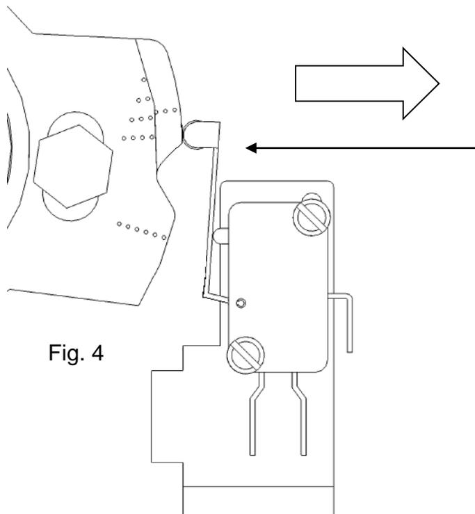
Ensure the switch lever closes the contacts, if not adjust by bending the lever arm towards the cam.
