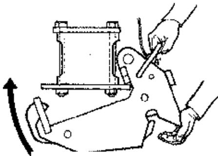
3. Fit lift-in hitch assembly
