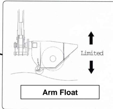
This is only to be used in verge mowing set up, it will reduce weight on the rear roller allowing head to move more easily, following small changes in ground contours in a forward motion, with the aid of a pre-charged gas accumulator.
