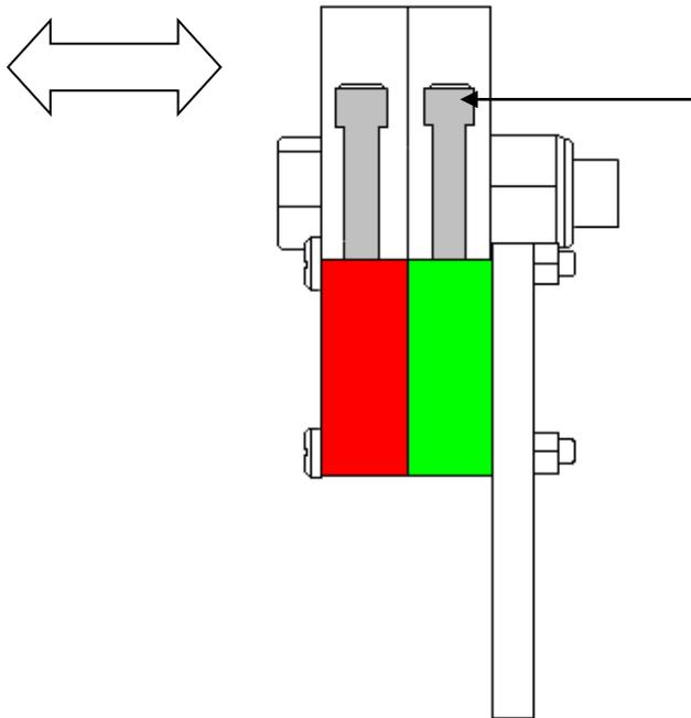
Bend lever arm of switch to align with the middle of each cam, ensure they don't overlap onto the adjacent cam.
