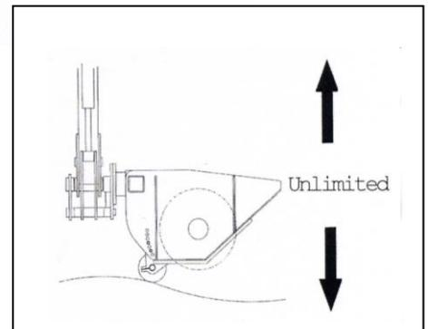
Autopilot will only operate when the cutting head rear roller is in contact with the ground.
