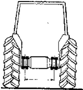
1. Mount axle brackets as instructed on separate fitting sheet specific to your tractor type.
