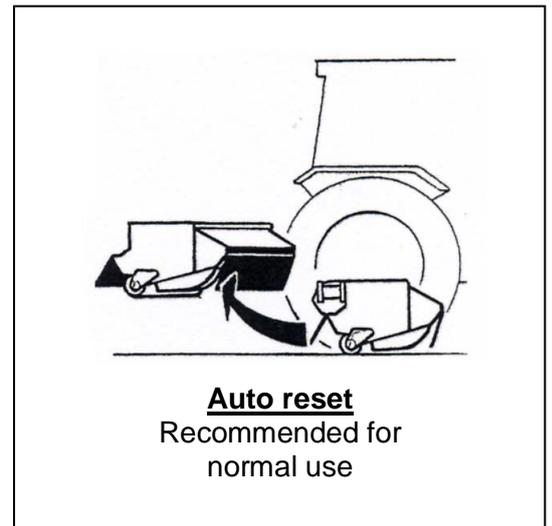
**Never attempt to operate the machine when travelling backwards, the break back will not function and any damage caused will not be considered warranty. The break back feature does not excuse the machine operator of their need to be aware of obstacles and to avoid hazards. It is your responsibility to maintain a long reliable working life.**
