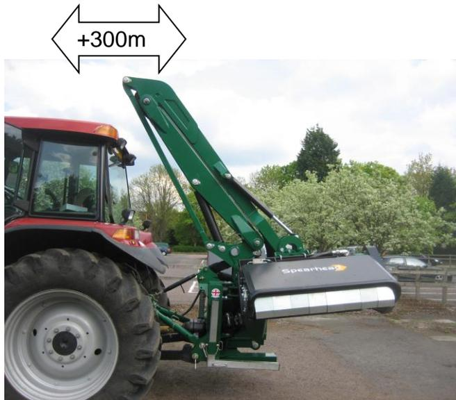
4. Carefully position main boom over the tractor cab roof until rubber bump stop meets the flip-over transport bracket, allow minimum of 300mm.
