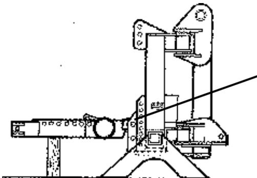
4. Assemble sub frame to suit axle width 1m or 1.1m, mount sub frame assembly to your machine using bottom pin holes.
