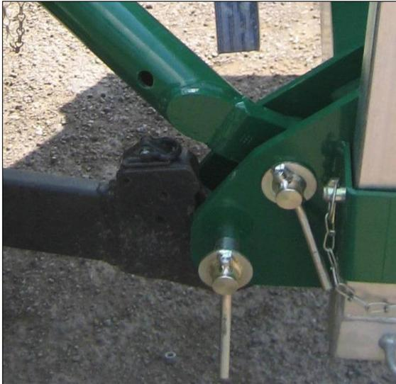
1. Reverse tractor to machine and attach lower links.
