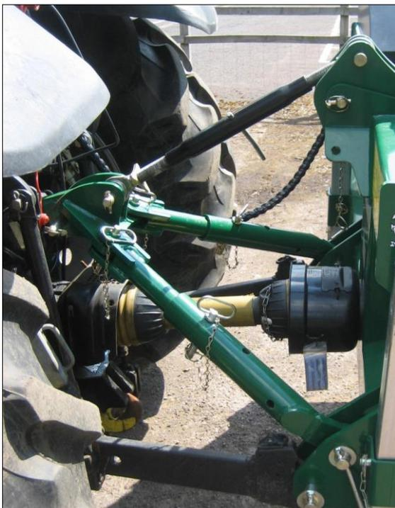
3. Fit stabiliser tubes between A frame and stabiliser bracket. Ensure the tubes are free to slide, do fit locking pins.
