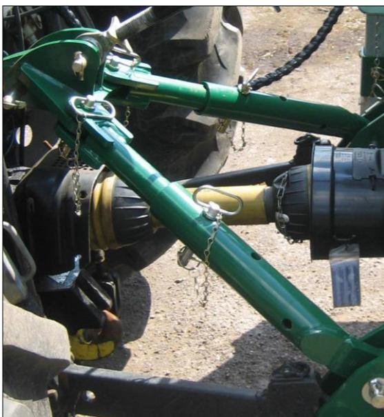
6. Fit locking pins to stabiliser tubes, then the linkage can be lowered so that the weight of the machine is taken by the stabilisers. It is essential that both tubes are set to equal lengths, more than one attempt may be required to achieve the correct height as the machine settles on the stabilisers.
