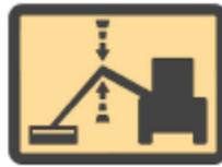
This is only to be used in verge mowing set up, it will reduce weight on the rear roller allowing head to move more easily, following small changes in ground contours in a forward motion, with the aid of a pre-charged gas accumulator.
